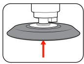
4. To remove the sand paper, peel off starting from one edge.
