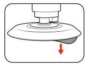
Note: Before operating, ensure the counter weight is rotated out of the way so that the spindle is free to spin.
