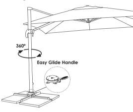
Step 10: When not required, use the crank to wind the canopy down. Press the trigger in the easy glide handle and move the handle to the bottom position.
