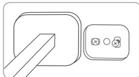
**TIP:** For towel rails, determine the centre positions for the mounts using the right (or left) hand sides of the rail base.
