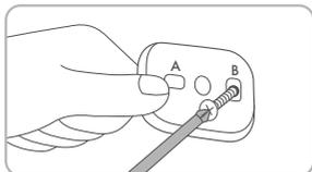
Using the screws provided and a phillips head screw driver, fasten the mounting plate horizontally on to the wall.
