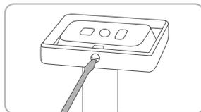
Remove the mounting plate from the bathroom accessory being mounted, by unscrewing the lug at the base with a small flat head screwdriver.
