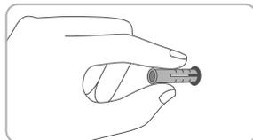
Drill a 5mm diameter hole into the wall surface using a suitable drill bit (eg tile or masonry) and insert the wall plug provided.
