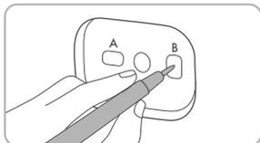
Position the mounting plate on the wall and mark the centres (positions A and B) noting that this plate can be easily adjusted to achieve a horizontal alignment. These holes should be 22mm apart.
