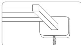
Position the accessory over the mounting plate and tighten the lug screw with a small flat head screwdriver.
