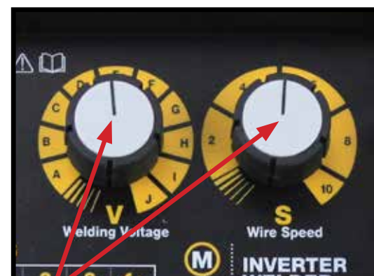
15 Set The welding Voltage and Wire Speed according to chart
