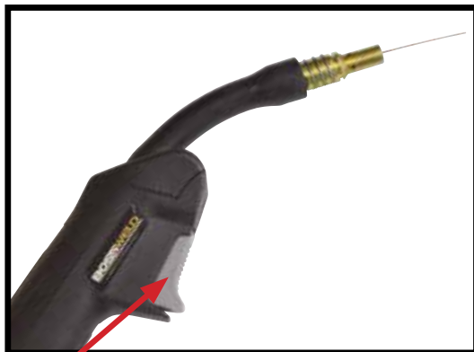
11 Press the trigger. This will feed the wire through the torch. Release button when wire appears at the end of the torch. NOTE: Make sure your torch is layed out straight
