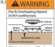
Fill fuel only to bottom of fill neck. Expansion of fuel from heat of sun or normal operation may cause tank spillage if overfilled. Wipe up fuel spills and allow to dry before starting
