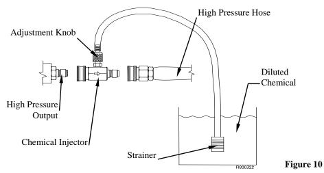
4. Submerge the suction strainer connected to the braided chemical hose into a bucket containing the chemical solution. See Figure 10.
