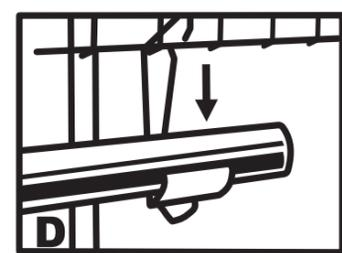
After expanding Clothes Rod to desired length, place into Hanging Rod Brackets and press down to snap into place.
