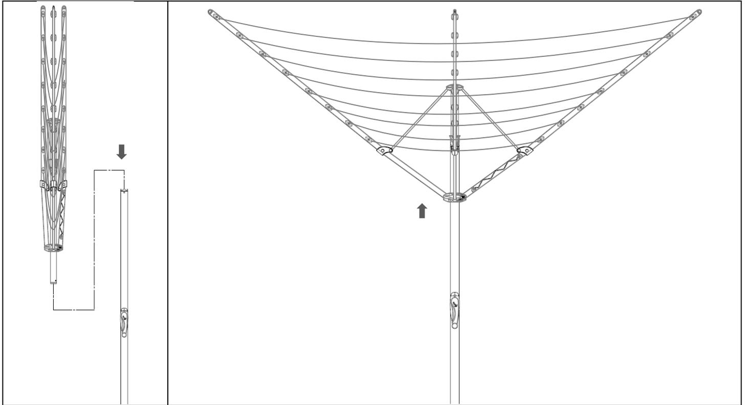
**Note: Once the Arm Assembly is connected to the Main Post it cannot be removed.**
