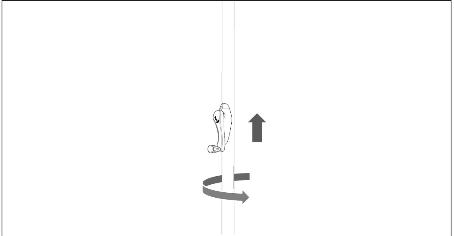
Your clothesline can be removed from the ground socket for storage. The Main tube locks to the ground socket for safety
