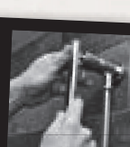
Push in rail and tighten with pin lever
