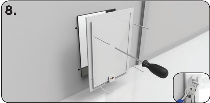
8. Screw inner door frame into door/panel. Tighten with a Phillips head screw driver. If screws protrude trim the ends to be flush.
