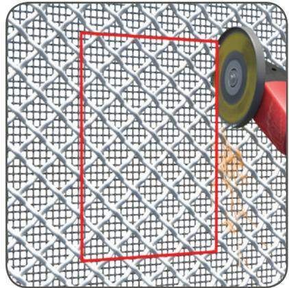
1. Take the measurements needed to cut the opening by following steps 1-3 of the previous instructions. Using an angle grinder, cut out the opening.
