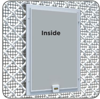
4. Screw inner door frame into security screen.
