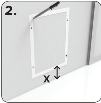
2. Cut out template supplied in box, line up bottom of cut out with height (x) and trace onto door. Mark screw hole positions as well.
