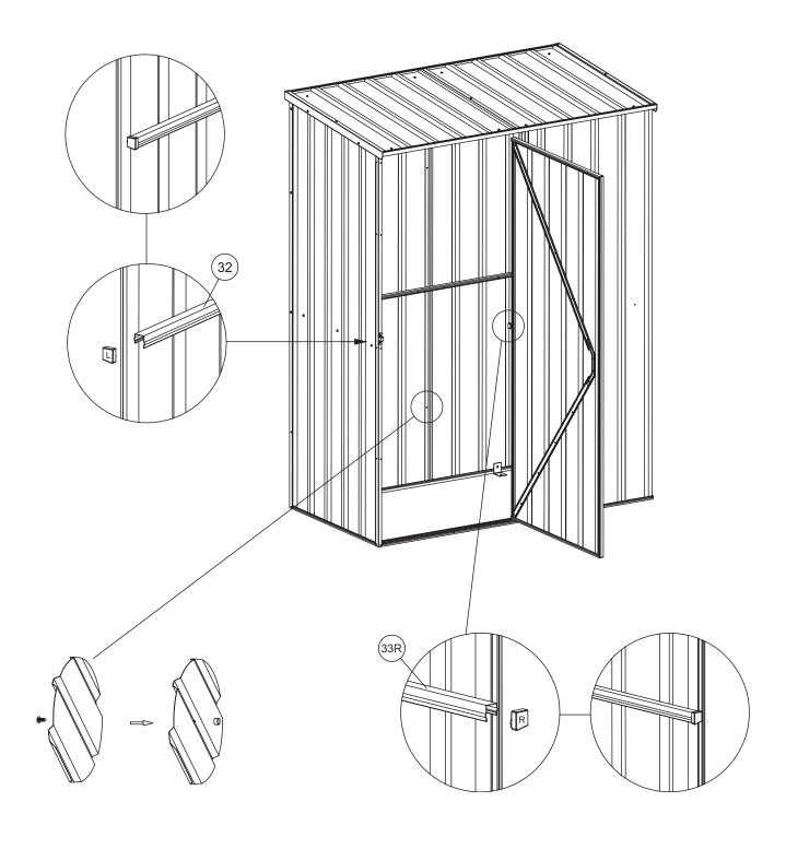
The door can be hinged on the opposite side as well. Align the door with the edge and make the holes using a cordless drill.
