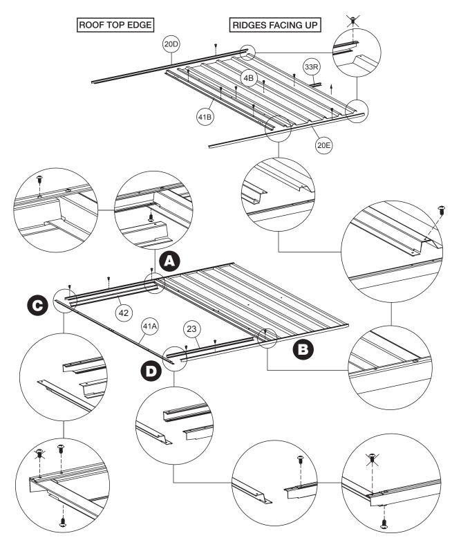
Fit part 41A (jamb), part 42 (jamb) and part 23 (bottom channel) and fix them with self-tapping screws - except those marked with a cross. Make sure both joins (diagrams A and B) are fixed the same followed by diagrams C and D.
