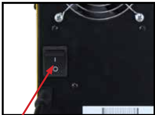
10 Plug machine into 240V and switch to the ON position on the back of machine.
