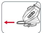
2 Align the tabs of the safety guard with the recess in the back of the cutter head.
