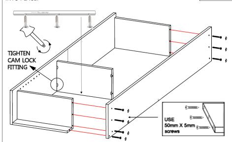
INSERT YOUR 4 PINS (9) INTO THE HOLE NO: (8) PROVIDED. INSERT THE CAMS INTO THE HOLES PROVIDED ON THE BOTTOM OF THE SHELF. USING SCREW DRIVER TWIST CAM INTO LOCK POSITION.
