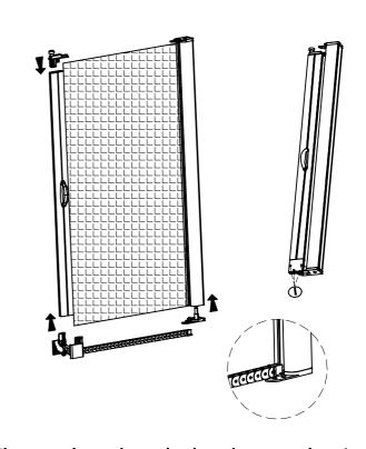
Then put the end caps back to the screen housing + handle profile, assemble again.
