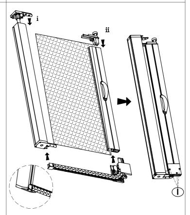
Then put the end caps back to the screen housing + handle profile, assemble again.
