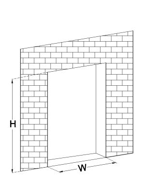
Measure the dimension of the door ( High and Width), then cut the profiles as following
