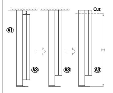
Then make the end of both profiles on the same level for cutting.
