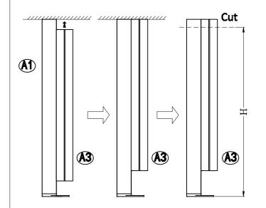
Then make the end of both profiles on the same level for cutting.
