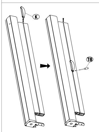
After cutting, put the handles into the handle profile and fix it to the proper position.
