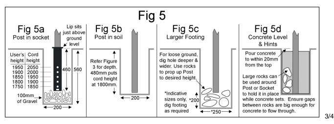
**1.** Mix concrete in the ratio of 4 gravel, 2 sand and 1 cement or simply use premixed concrete packs. To hold the Post/Socket erect, the concrete must be mixed fairly dry but should still be wet enough that it sticks to itself when squeezed in the hand, it should not crumble.
