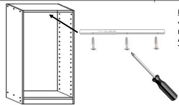
YOU WILL NEED TO RETRIEVE THE INFILL FROM PART 2, USING 3 X 30mm SCREWS PROVIDED, ATTACH THE INFILL TO THE UNDER-SIDE OF THE FIXED TOP SHELF.
