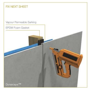
Once both sheets are fixed, check the joint for gaps and fill with additional sealant if required.
