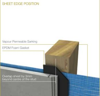
Position the underlap sheet on every stud 3mm past the centre of the stud to ensure the fasteners fixed at the edge of the sheet have adequate distance into the stud.
