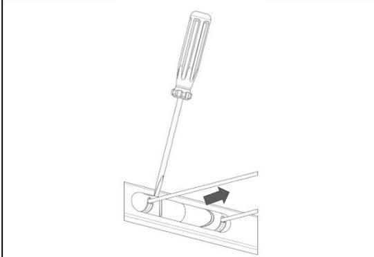
Use a flat bladed screwdriver to unclip the Line Hook Cover from the arm
