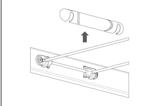
The Line Hook Cover has slots so it can be lifted upwards without removing the line
