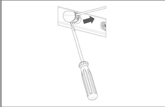
Use a flat bladed screwdriver to unclip the Tensioner Cover from the arm.
