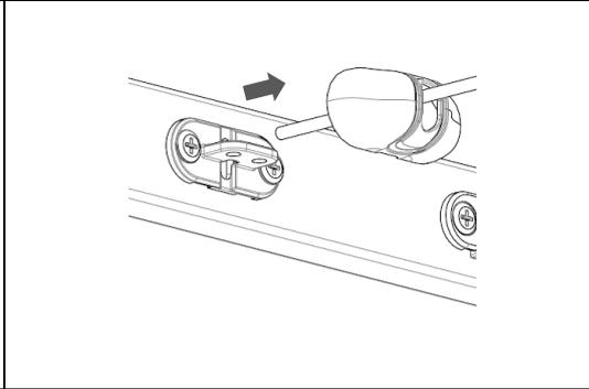
Unthread the line and remove the Tensioner Cover.
