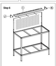
Place tool tray 'I' against the pegboard and secure with bracket 'J' and 'K'.
