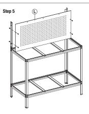
Put pegboard 'L' in place and fasten nut and bolts. Once in place tighten nuts and bolts.
