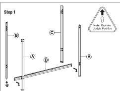
Place foot end caps onto the bottom of the legs 'A', 'B' and 'C'. Note upright position. Place shelving brackets 'D' onto the legs. A rubber mallet can be used to lightly tap all brackets into the keyholes of the legs into place.
