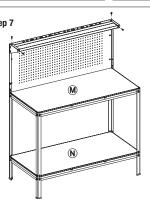
Fasten brackets onto tool tray with the supplied bolts and place bottom shelf 'N' followed by
