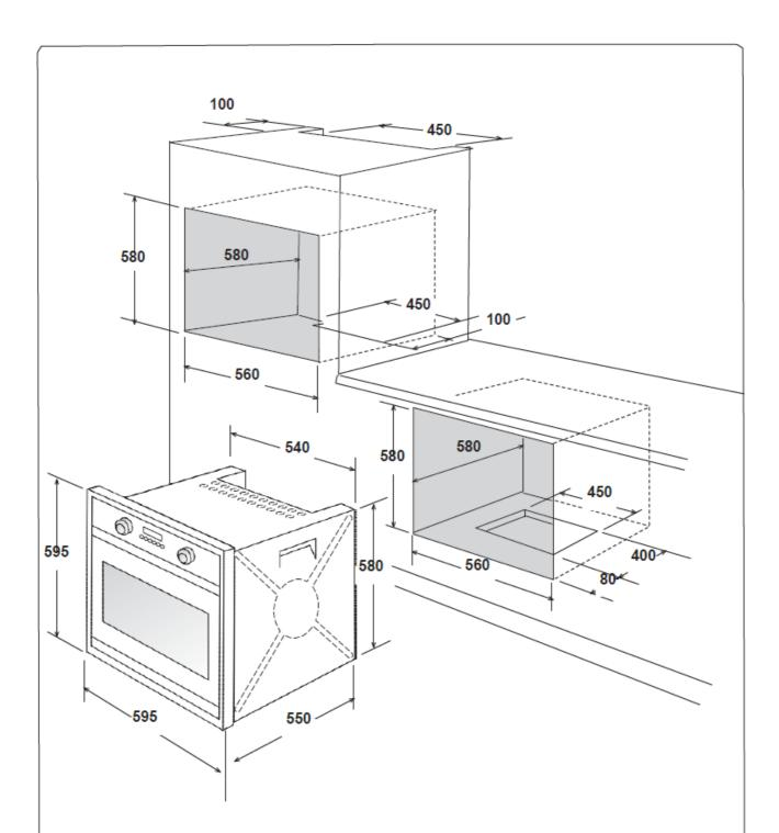
Cabinetry materials must be suitable to withstand temperatures up to  $90^{\circ}\text{C}$
