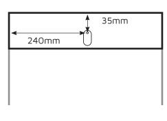
NB: If using the upgraded LED hang rail, DO NOT cut through the LED light –cut either side of the light to ensure correct operation.
