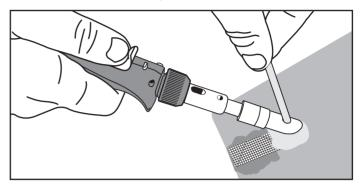
Remember that you can stop and repair and then recommence at any time. This is a heat based process. You are not dependent on any chemical curing so you can stop and start when convenient.
