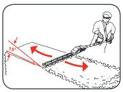
**Note:** Do not use the pole hedge trimmer for cutting stems greater than 12mm. Use the trimmer only for cutting normal shrubbery found around houses and buildings.
