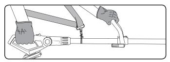
Slide the switch lock (a) to the front with your thumb and hold, then squeeze the trigger switch (h)
