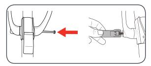
Select the most comfortable position and close the lever to lock the auxiliary handle in position.
