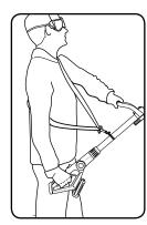
• Trimming new growth. Using a wide sweeping motion, feed the blade teeth through the twigs. A slight downward tilt of the blade, in the direction of motion gives the best cut.
