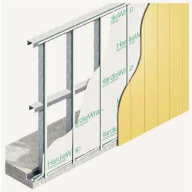
Installation of HardieBreak™ thermal strip for flat sheet direct fix
