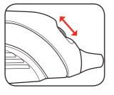
Note: The higher the number on the variable speed dial the faster the oscillation frequency of the multi function tool.
