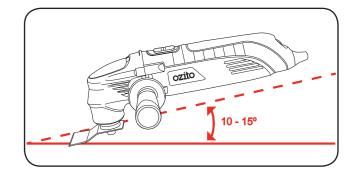
3. Allow the scraper to do the work; do not apply heavy pressure to the multi function tool. This may cause the multi function tool to overload or cut into the surface of the workpiece.
