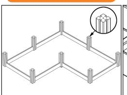
Select your required design. Remove posts & attach discs (ensuring you have the 8mm holes on top) then slide in the first row of non-branded boards by holding each end and applying equal force downwards.Slide in the remaining boards on all external sides ensuring the Birdies branded board is located in the top row.
