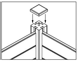
Insert the 4 hardwood dowels into the holes on the top of the posts by hand and then place 4 caps over these dowels. Push down to secure. **OPTIONAL** Wood glue can be used to fix the cap in place.
