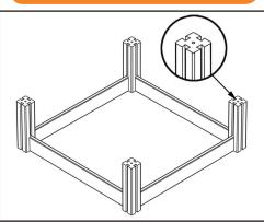
Remove posts and attach discs, ensuring the 8mm hole is on top and slide in first row of non-branded boards by holding each end of the boards and applying equal force downwards.
