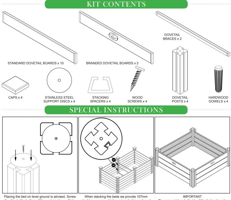
Placing the bed on level ground is advised. Screw the disc to the bottom of the post as shown. Note the larger 8mm hole is the top of the post. The disc is not required on hard level surfaces such as concrete, deck or pavers
