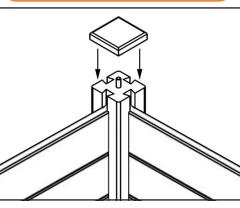
Insert the 4 hardwood dowels into the top of the posts and then place 4 caps over these dowels and push down to secure. OPTIONAL: Wood glue can be used to fix the cap in place
