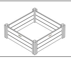
Slide in remaining 8 boards ensuring the Birdies Wood Branded board is located in the top row.
