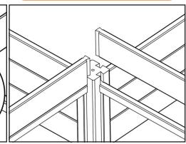
Slide in a first row of non branded boards, placing them onto the top brace.
