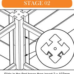
Slide in the first brace then insert 2 x 107mm stacking spacers in each post. Slide in the second brace until it rests onto the spacers.
