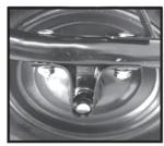
**Step 11:** Tighten all nuts securely. Inflate the tyre to a maximum 25PSI. Please ensure you use a manual pump to avoid injury and do not over inflate.
