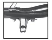
**Step 10:** Slide the axle (J) through the wheel (K) and insert into the fixed axle bracket. Using medium bolt (M) secure the other axle bracket (I) into position with spring washer, washer and nut.
