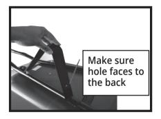
**Step 5:** While holding the wheelbarrow tray on its side, remove the nut from the bolt inserted in step 2. Then insert the long bolt (N) through the tray, handle and leg and secure using a spring washer, washer and nut. Repeat on the other side.
