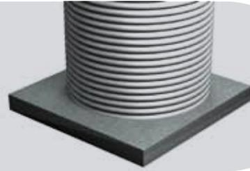
A concrete slab base is the most suitable base for your Aquaplate® rainwater tank. Construction of a concrete base needs a minimum of 100mm thick concrete and F62 mesh, on a flat level area. If the tank is to be positioned in an area that is on a slope then the thickness of the slab is to be increased and the mesh to be a higher grade. The slab must be flat, smooth and level. Finish with a metal trowel is advisable.
