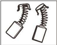
When the carbon brushes wear out, the drill will spark and/or stop. Discontinue use as soon as this happens. Carbon brushes should be replaced prior to recommencing use of the drill. They are a wearing component of the drill and therefore not covered under warranty. Continuing to use the drill when carbon brushes need to be replaced may cause permanent damage to the drill. Carbon brushes
