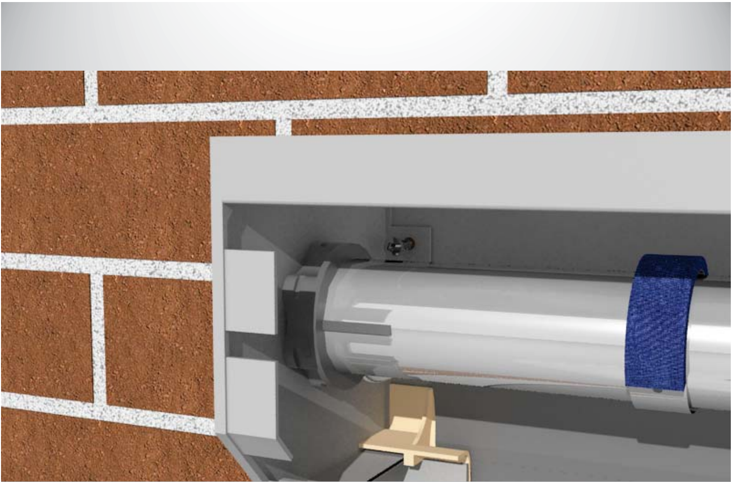
27. With the shutter out of the way, secure the pelmet box on the wall.
