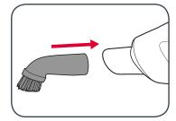
2 To remove simply pull the accessory away from the vacuum nozzle.
