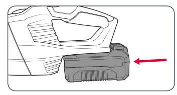
2 To remove, press and hold the battery release tab and pull the battery away from the vacuum.
