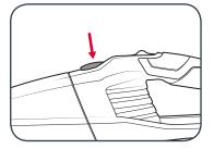
2 Remove the debris container by pulling the top of the container away from the vacuum housing.
