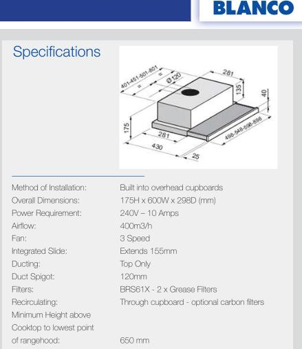
NOTE: Measurements are within 2- 3mm factory tolerance. It is advisable to check dimensions of physical product when measuring for installation and before doiung any cut outs.
