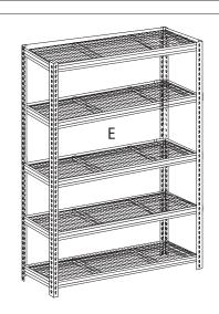
Step 5: Lay the Wire Shelving (Part E) between the Beams as shown.
