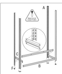
Step 1: Assembling bottom of frame
