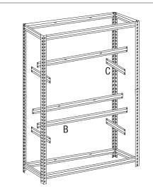
Step 3: Assemble remaining shelving Assemble remaining Short Beams (Part C) and Long Beams (Part B) to your desired shelf height. As before, lock rivets to the bottom of the keyhole by tapping the Beams with a rubber mallet.
