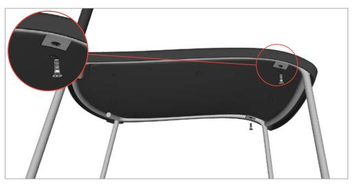
**STEP 2:** Fully tighten seat shell to chair frame with provided screws.
