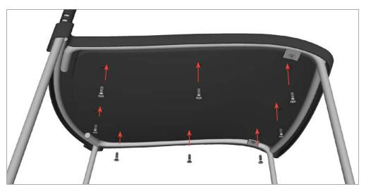
**STEP 4:** Fully tighten seat shell to chair frame with provided screws.
