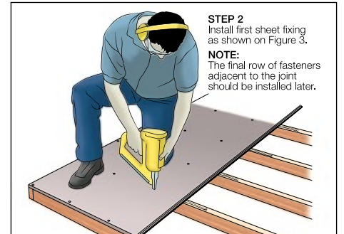
FIGURE 4 FIXING 1ST PANEL
