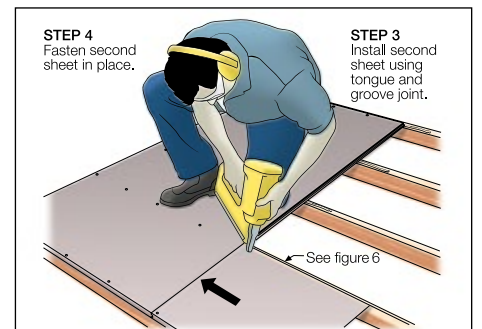
FIGURE 5 FIXING 2ND PANEL
