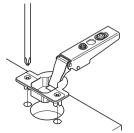
Cup fixed with pre-mounted spreading dowels.
