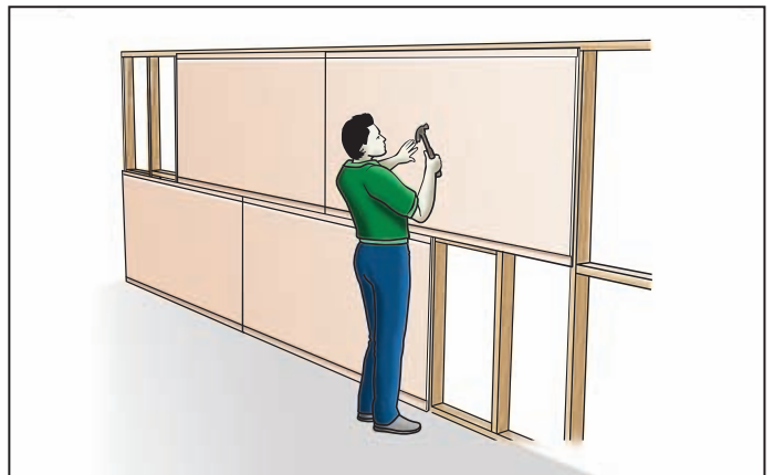
FIGURE 5 FIXING REMAINING SHEETS
