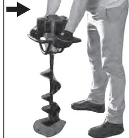
**CORRECT OPERATING POSITIONS IS WITH POST HOLE DIGGER HANDLES BELLOW WAIST LEVEL**
