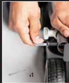
Then, carefully fully tighten the bolts onto the bracket by using the installation T40 wrench. Try to keep the bolt in the handles directly in line with the holes in the bracket as much as possible when tightening.
