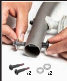
Push the bolts through the holes located on the lower half of the handles, ensuring that a washer is in between the handle and the bracket on the Mower. Insert the bolt through the hole and into the bracket on the mower on both sides prior to tightening.
