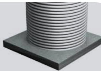
A concrete slab base is the most suitable base for your Aquaplate® rainwater tank. Construction of a concrete base needs a minimum of 100mm thick concrete and F62 mesh, on a flat level area. If the tank is to be positioned in an area that is on a slope then the thickness of the slab is to be increased and the mesh to be a higher grade. The slab must be flat, smooth and level. Finish with a metal trowel is advisable.
