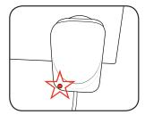
With the battery sitting on a flat surface, align the raised ribs on the battery with the recess in the charging cradle and slide onto the battery ensuring a firm connection.
