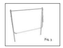
4) Remove the left and right side arms from the clothesline box and position near the appropriate Post. N.B. *The bent side arms should face toward each other (Fig. 3).*
