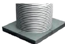
water to set the sand and cement off. Paver base is to be large enough to support all edges of the tank. Tank may be placed on to paver base straight away. Do not fill tank above 2 corrugations for at least 48 hours.
