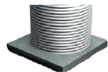
Slabs must be large enough to support all edges of the tank, and should be at least 100mm longer and wider than the tank. Slabs must be allowed to cure for at least five days prior to placing tank on slab.
