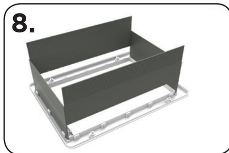
8. Fit all 4 partitions into outer door frame. Optional: Use duct tape to secure the corners of the partition to each other for easy installation.
