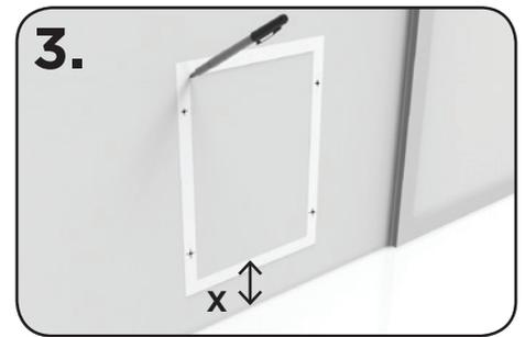
3. Cut out supplied template, line up height (x) with opening & trace on to door.
