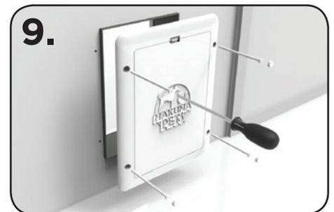
9. Screw into door from inside. Place nut over screw ends, cut off excess plastic screws. Optional: seal around frame of pet door with silicone.
