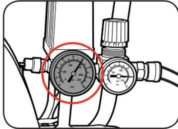
**Note:** When the maximum preset tank pressure is reached, the motor will automatically switch Off. As the compressed air is used, the pressure will drop until it reaches the preset minimum pressure, when the minimum pressure is reached the compressor will turn on again automatically to build up/maintain pressure.
