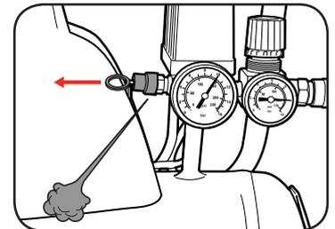
3 When the ring on the safety valve is released the air discharge should stop.
