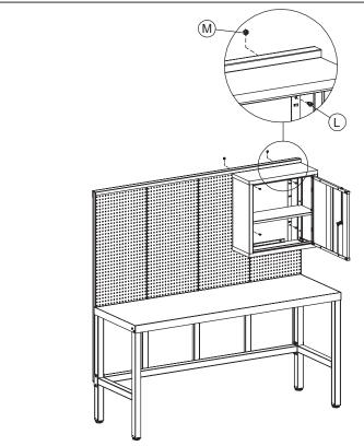
Step 5: This cabinet can be easily mounted onto a peg board (see Pinnacle Hardware item GOS025 from our Garage Storage System) using the included Phillips-head bolts (L) and hex nuts (M) as shown in the diagram above.
