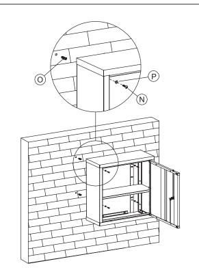
Alternatively, the cabinet can be mounted onto a wall. First, drill four holes which align exactly with the holes in the back panel for mounting the cabinet. Then insert the included plugs (O) into the holes and use the long self tapping screws (N) and washers (P) to attach the cabinet to the wall.
