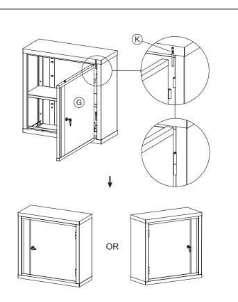
Step 4: Install door (G) by aligning door hinge slots with those on right side panel (C) and insert hinge pins (K).
