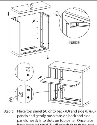
have been inserted, fix all panels together using self tapping screws (J) as per diagram above. Install shelf supports (H) into slots in all four corners at an even height and insert shelf (F).
