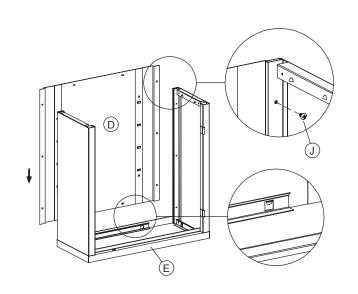
Step2: Slide back panel (D) into bottom panel (E) ensuring tabs on back panel insert into slots in bottom panel. Then attach back panel (D) to side panels (B & C) using self tapping screws (J) as per the diagram above.
