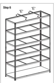
Apply remaining brackets as above to desired height. Ensure that braces 'E' are fixed to all shelves.
