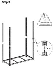
Place MDF board on bottom shelf to minimise buckling. Join the upper legs to the lower legs with the connector pins.
