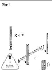
Place foot caps onto the bottom of the 4 legs 'F'. Note upright position. Place shelving bracket 'C' onto the legs 'F'. A rubber mallet can be used to lightly tap all brackets into the keyholes of the legs into place. Allow one keyhole free between the foot cap and the shelving bracket.
