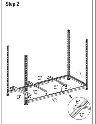
Use shelf bracket 'D' for the side brackets using the shelf bracket from Step 1 as a guide for height. Allow 1 keyhole free from the ground as shown in the diagram. Use same shelving brackets for opposing sides as shown in the diagram. Place brace 'E' as shown.
