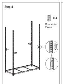
Join the top rivets of the connector plates to the bottom keyholes of the upper legs and bottom rivets of the connector plates to the top keyholes of the lower legs. Gently tap the connector plates in place with a mallet and a screw driver on the notch.
