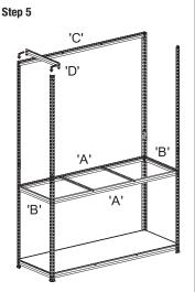
Fix brackets 'C' at the very top allowing room for the MDF board to sit flush against the legs. Repeat with brackets 'D'.
