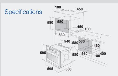
Product Dimensions: H595 x W595 x D550mm Cut-out size (proudmount): H580 x W560 x D580mm Cut-out size (flushmount): H598 x W598 x D580mm 220-240V - 50Hz
