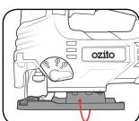
4 Once the angle is correct, slide the shoe forward for the pin to make contact.
