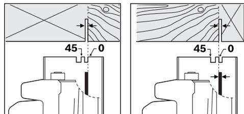
The 0° cutting mark **9** indicates the position of the saw blade for right-angled cuts. The 45° cutting mark **8** indicates the position of the saw blade for 45° cuts.
